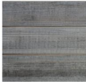
Graphite weathered after 6 months
